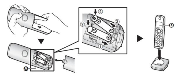
**Note:** If the batteries are fully charged, but the operating time seems to be shorter, clean the battery ends (+,-), and the charge contacts with a dry cloth and charge again.
