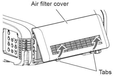
Pull out the air filter cover from the hook of the projector while slightly pushing upward the tabs of the air
