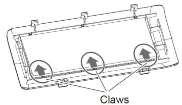
Please make sure that there is no damage or deformation at the contact areas of the pre-filter with the claws when attaching it.
