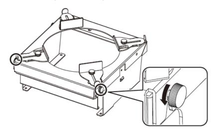
3. Remove the lens fixing attachment bracket as shown in the figure.
