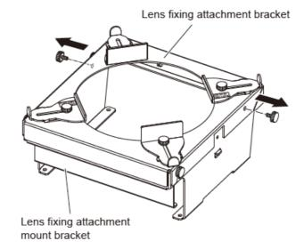
2. Loosen the two lower thumbscrews (inserted in slots).
