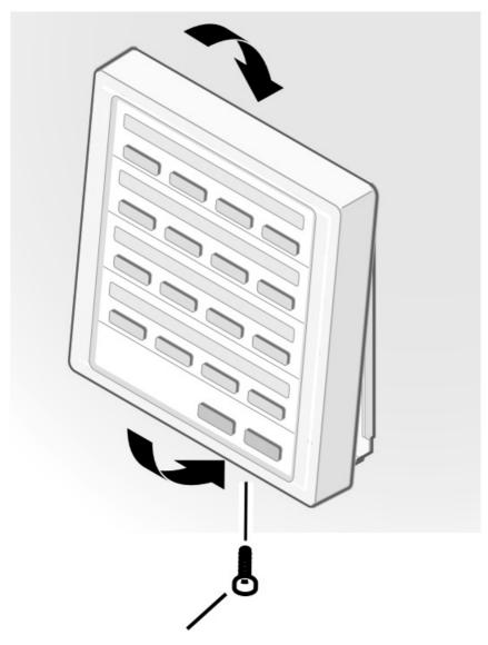
3 Attach the screw for fixing the control panel.
