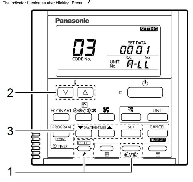
1. Press and hold the 3 buttons for 4 seconds or more simultaneously.
