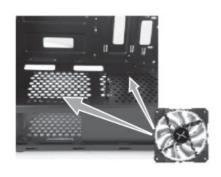
PUT 2×120MM FANS ON THE PSU COVER 2.5" 5SD INSTALLATION
