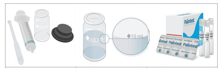
Rinse equipment thoroughly with d eionised water or the water being t ested.
