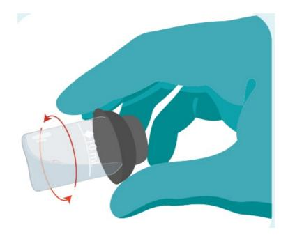
Align tubes as shown. Always use the tube cap as it excludes light from the optics.
