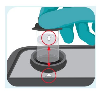
Keep instrument clean. Dry all tubes before placing in the optical cell.
