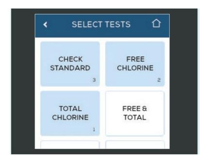
Highlight test types by pressing them. A number appears in the bottom right corner. The number represents the order in which they appear on test selection screens.
