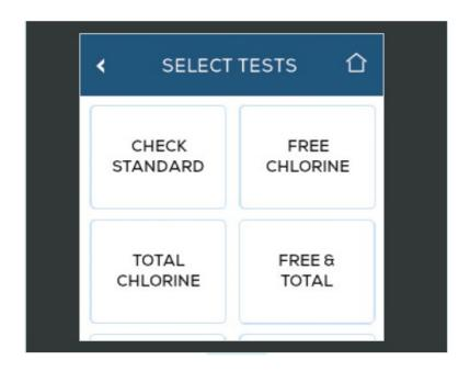
Press the back button to return to the CONFIGURATION menu. It is not possible to navigate away from the screen without at least one test type selected.
