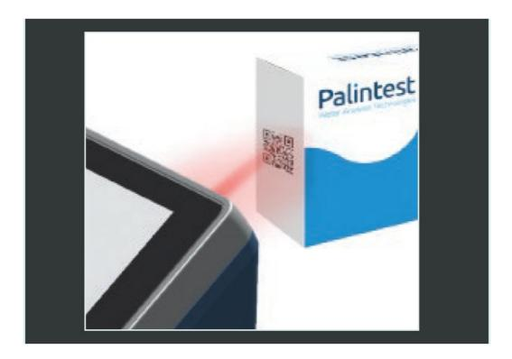
Scan the QR code on the side of the box of sensors. Details about the batch will appear in a notification on the screen and automatically sorted into the correct folder. If a batch is added as a duplicate, the "loaded on" date will update but nothing else will change.
