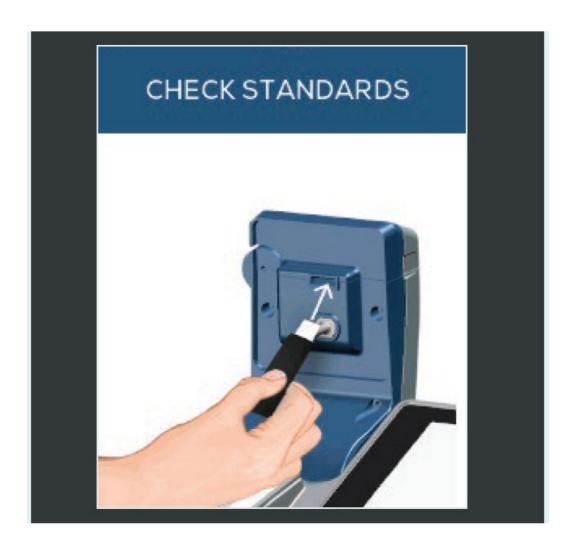
Open the arm, and insert the first of three check standards from the KEMC10 pack.
