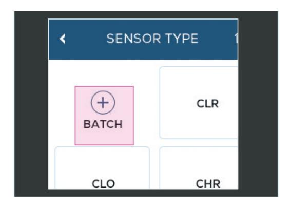
Select the sensor type code from the list. The code is also the start of the batch code and can be found on the foil packaging or box.
