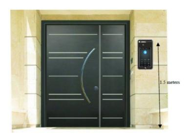
The recommended installation height for the camera is 1.5 meters (4.9 feet) above the ground.
