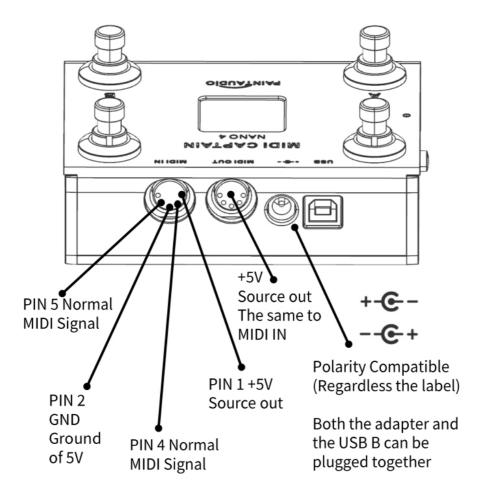
The 5V special power output on PIN 1 may conflict with custom power outputs from other devices. To avoid this issue, you can use a MIDI cable with only PIN 4 and 5 connected (our cables are designed this way)
