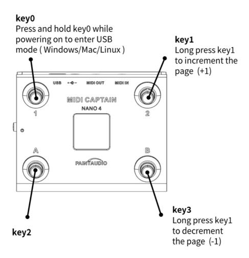
This picture is representing the correspondence between key customization settings in USB mode and the actual physical keys
