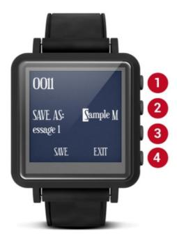
To save the message for that key, use the button 2 and button 3 arrow keys to select "Save" and press the button 4 key to confirm. A display screen will show "OK" and will revert back to the pairing screen. Repeat previous steps to program additional keys of the same call button or different call button keys. To exit the pairing screen, press the 1 button.
