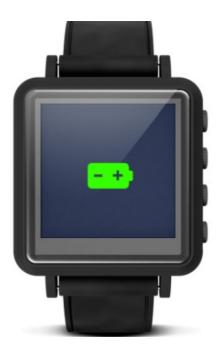
Ensure that your watch is dry and there are no obstructions on the charging pins. Please allow your pager to be connected to the charger for 30 minutes to 1 hour for a complete charge.
