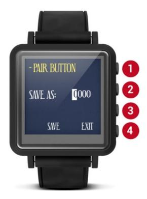
Press the key on the Onyx Call Button that you wish to pair to the Wear & Go Watch. When the Wear & Go watch receives the signal from the call button it will show a 4 digit identifier number on the top left side of the display.
