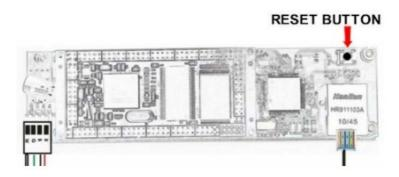
In case the password and network setting have been forgotten, reset the password and the network setting to factory default. Follow the steps below
