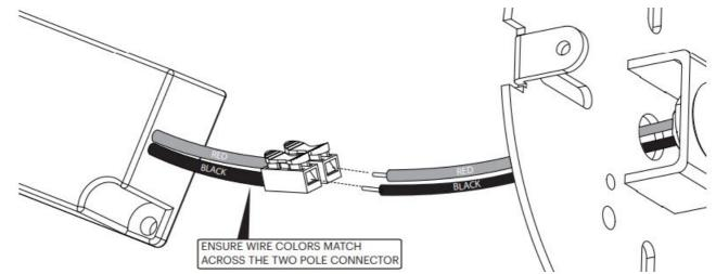
3. TUCK TRANSFORMER AND WIRING INTO JUNCTION BOX AND SCREW MOUNTING PLATE INTO JUNCTION BOX USING PROVIDED MACHINE SCREWS
