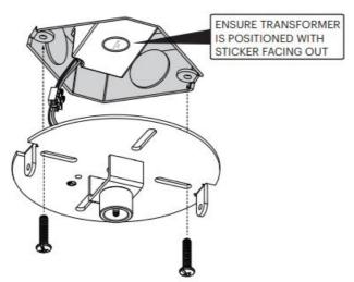
4. FASTEN CANOPY COVER TO MOUNTING PLATE USING PROVIDED MACHINE SCREWS
