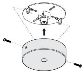
5. HOLD OUTSIDE OF SHADE WITH BOTH HANDS AND SCREW FIXTURE HEAD INTO CANOPY ASSEMBLY
