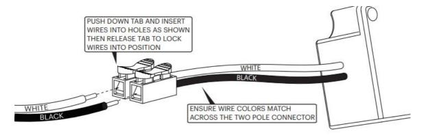
2. CONNECT FIXTURE WIRING ON MOUNTING PLATE TO 2 POLE CONNECTOR ON DC OUTPUT SIDE OF TRANSFORMER
