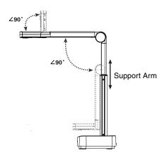
\*\*Please only operate in the extended angles as illustrated. Improper usage may damage the machine.
