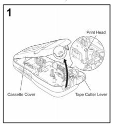
2. When replacing batteries or tape cassettes, make sure the power is turned off.
