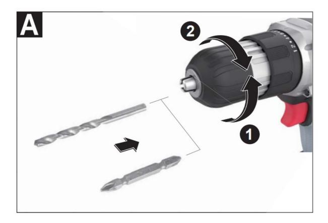
Open the keyless chuck by turning in rotation direction **1**, until the tool can be inserted. Insert the tool. Firmly tighten the collar of the keyless chuck 2 by hand in rotation direction **2**. This automatically locks the drill chuck.
