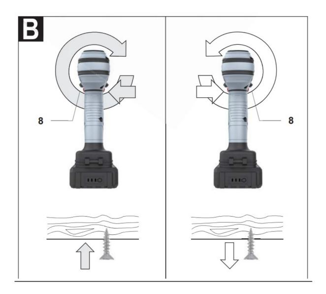
Rotate clockwise: Move the rotational direction switch on both sides up to the stop into position
