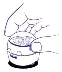
3. Bit+ will move and blink green. That means it's calibrated! If Bit+ blinks red, start over from step 1.
