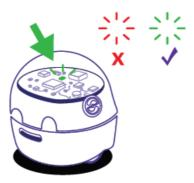
4. Press the Go button to turn Bit+ back on.
