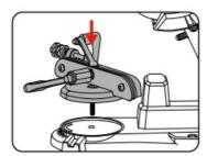
• Secure the table in place by fixing the locking knob to the bolt (by screwing the knob clockwise).
