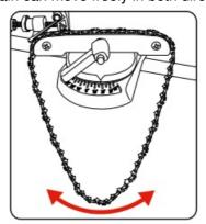
• If you know the angle of the chain, rotate the table to the same angle as the chain. To rotate the table loosen the table lock knob and rotate the table until the scale indicator lines up with the scale on the base of the sharpener.
