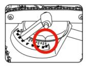
• Take hold of the hand piece and bring it down so that the wheel is slowly lowered into the chain, along the cutting tooth. Slowly move the table so the cutting face of the tooth is parallel with the edge of the wheel. The most common chain angles are 30 – 35°. It may be necessary to slide the chain slightly to allow the wheel to enter down the face of the tooth.
