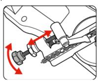
• When the chain stop is properly adjusted it should be directly behind the chain tooth as shown. To secure in position rotate the chain stop lock nut clockwise as far as possible.
