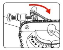
• Adjust the chain stop knob so that it is firmly behind and at the bottom of the aligned chain tooth, by rotating either clockwise to move the chain stop forward or anti-clockwise to move the chain stop backward.
