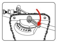
• Should the chain still not be clamped, pull the clamping lever outwards (away from the guide), turn the lever anti-clockwise 1/4 of a turn. Push the lever back in towards the guide. Proceed to rotate the lever fully clockwise. Check the chain is clamped. Should it still not be clamped, repeat the process above.
