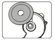
• Re-fit the locking knob and screw clockwise with the inside of the knob facing down against the sharpening wheel. Hold the wheel with the free hand to ensure the locking knob can be tightened properly
