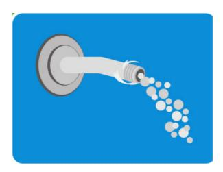
**STEP 3** Wrap plumber's tape clockwise3 or 4 turns around threaded end of shower arm.
