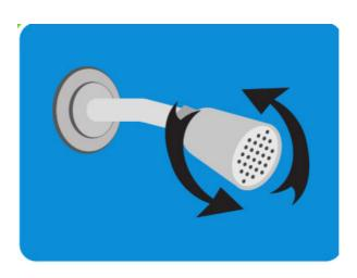
**STEP 2**Remove any remnants of old plumber's tape and flush out shower pipe for 5 to 10 seconds.
