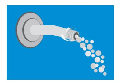
**STEP 3** Wrap plumber's tape clockwise3 or 4 turns around the threaded end of the shower arm.
