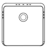
The Multi-sensor is used to measure the ambient temperature & humidity with built-in sensor and external temperature with remote probe. It is available to detect motion, vibration and allows you to receive notifications from mobile app. The above functions can be customized, please use this guide according to your customized functions. This guide will provide you with an overview of the product and help you get through the initial setup.
