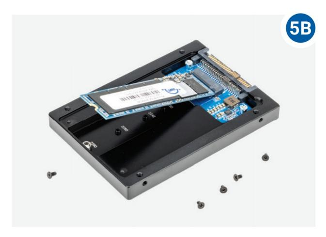
6. Hold the drive against its post, then use the drive post screw to affix the drive in place.
