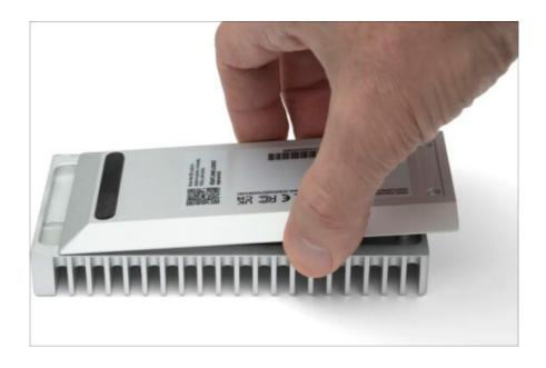
3. The drive post is pre-installed for a 2280 NVMe M.2 SSD. All other NVMe M.2 SSD form factors ( $2242 \mid 2230$ ) will need the drive post moved to the corresponding position.
