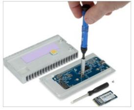
2. Carefully align the drive at a slight angle into the board connection and slide it forward until fully seated. Once the drive is fully seated use the included drive screw to secure the drive.
