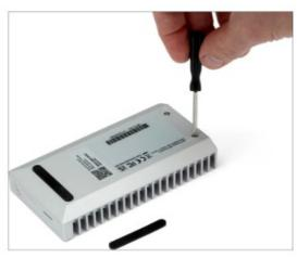
3. Peel the back of the rubber foot to expose the adhesive. Place and press the rubber foot into the notch housing the case screws.
