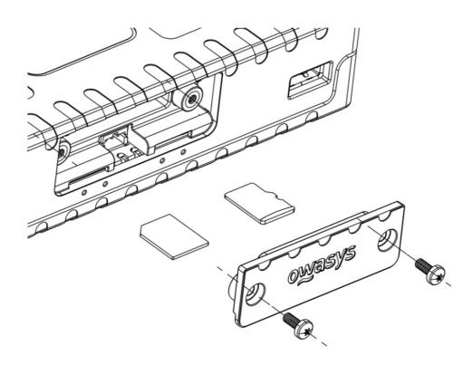
Then, insert the SIM card with contacts facing downwards as in the figure below. Same procedure for inserting the microSD card in its compartment and for connecting/disconnecting optional Battery using its one-position connector.
