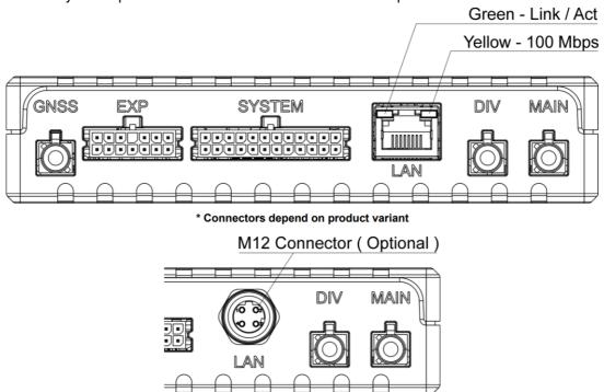
M12 Connector is an alternative to RJ45.
