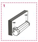
3. To mount the screen on the ceiling, hook the brackets. A suitable installation of the screen on the ceiling is presented in fig. 2.
