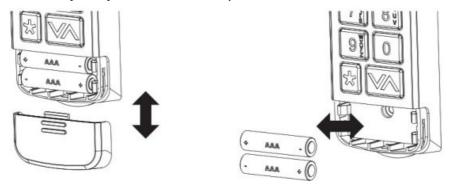
Use quality batteries. Do not mix old and new batteries. Do not mix alkaline, standard (carbon-zinc), or rechargeable (nickel-acmium) batteries.
