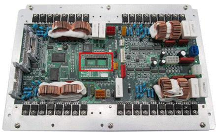
6. Remove the new EPROM from its packaging. Ensure the pins are aligned approximately 90 degrees perpendicular to the body of the EPROM (use a tabletop or similar flat surface, if necessary).
