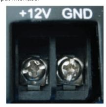
Adopt two sheath wires as connecting wires. Brown Wire to + Blue Wire to -
