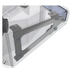
The rigging points consist of unperforated inserts designed to hold a M10 bolt. The inserts are made of anodized corrosion-resistant aluminium alloy (Ergal) but it is in any case suggested to protect against dust and any other external agents the points that are not used.
