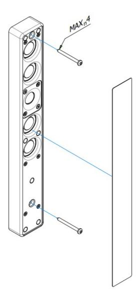
This system offers more than one way to install the loudspeaker as needed. To install the column either on wall or on a flat surface there are two through-holes dedicated as shown in the figure below. For this application, do not use screws with diameter greater than 4 mm. Proceed as follows:
