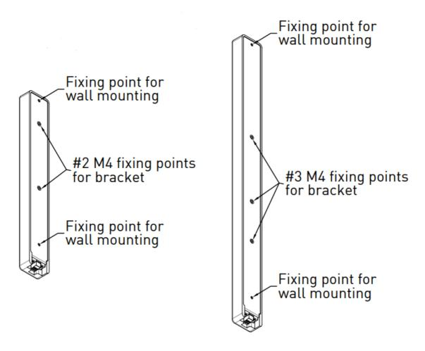
The AIWALL01 is a tiltable bracket for applications where a specific aiming is required or the surface does not allow wall mounting.
