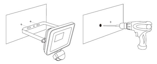
2. Step 2: Put expansion screws in the prepared mounting holes, then place the bracket in the mounting position and fix with screws.
