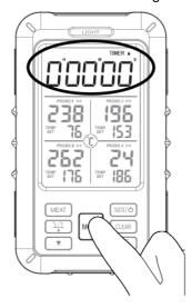
2. To start or stop the count up timer, press the START/STOP button when 0:00:00 is displayed on the monitor
