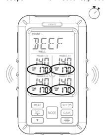
5. To turn off the alarm, press any key to stop the beep soud. This turns the orange light OFF and the blue light ON for 10 seconds. After 5 minutes it will re-beep once the temperature goes higher than the target set temperature. If the temperature is always lower than the set temperature, it stops alerting.
