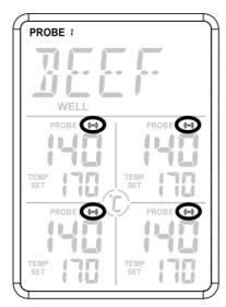
4. When the alert function is ON, it will signal an alarm once reaching the alert temperature, the alert icon will flash, the orange light will flash, probe 1 beeps for 1 second, and probe 2 beeps BIBI for 1 second, probe 3 beeps BIBIBI for 1 second, probe 4 beeps BIBIBIBI for 1 second
