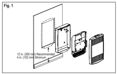
The hole must be 18 5/8 in. (473 mm) by 13 3/8 in.(340 mm); use the template printed on the cardbox of the heater.
