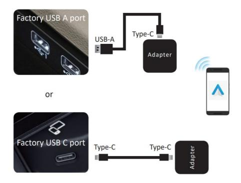
**NOTE!** The adapter should be plugged into the Android Auto-enabled USB port if there are multi USB ports in your car.
