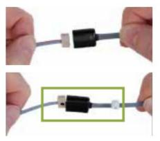
• Connect both plugs of the Y-cable of the Myo cuff to the free 3-pin sockets of the extension cable.
