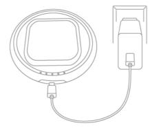
Stack batteries on charging base, lining up pogo pins to trigger flashing LED
