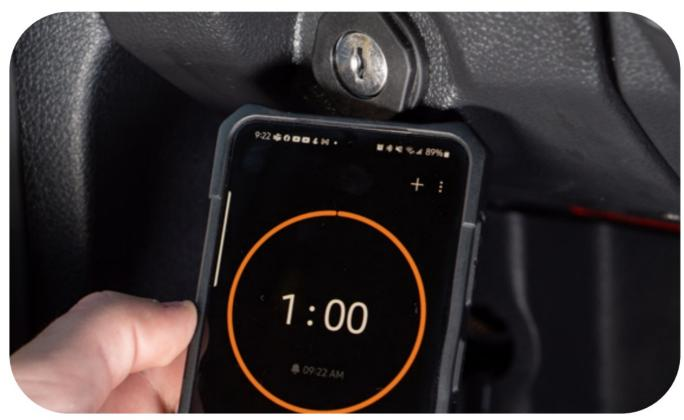
STEP 11 Insert the key and turn to the run position, but do not start the engine. Now the reset is complete.
