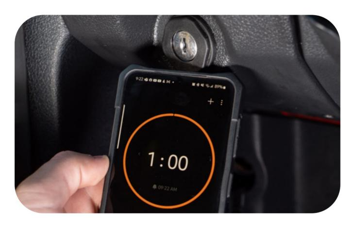
STEP 3 Insert the key and turn to the run position, but do not start the engine.
