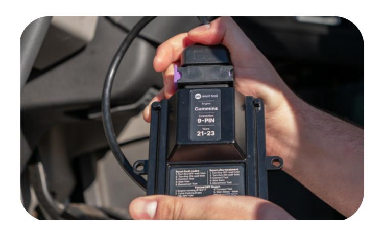
**STEP 6**Connect the adapter cable into the 9 pin diagnostic port of the truck.
