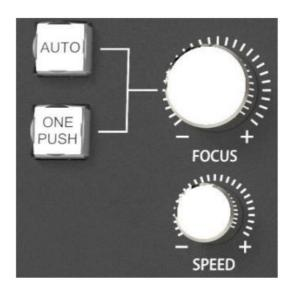
[AUTO] Button This lights in red when automatic adjustment of the focus is enabled
