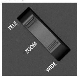
**[Zoom] Button** This a justs the zoom of a camera connected to the network. Press the [Tele] button to enlarge (zoom in), and the [Wide] button to reduce (zoom out)
