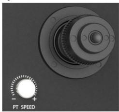
**[4D Joystick]** This controls the function of PTZ of each camera. Turn left or right for Pan control, turn up and down for tilt control. Turn the joystick clockwise to enlarge (zoom in), and counterclockwise to reduce(zoom out). Press the round button on top to for default setting of camera lens.
