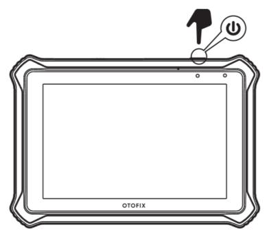
• Long press the Lock/Power button to turn on the key programming tool.
