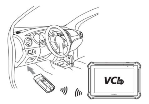
• Connect the VCI to the vehicle's DLC (OBD II port), which is generally located under the vehicle dashboard. Follow the on-screen instructions to connect the VCI to the OTOFIX IM1 key programming tool via Bluetooth.
