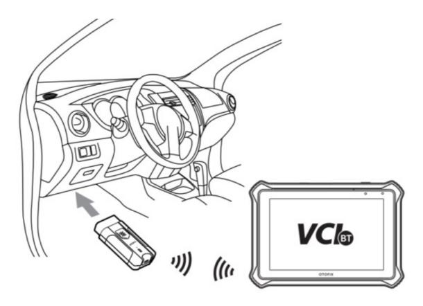
• Connect the vehicle and the key programming tool via Bluetooth or USB cable.
