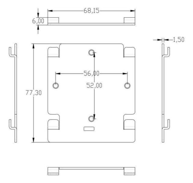
The bracket is fixed on the wall with 4pcs M3\*18 countersunk head tapping screws and 4pcs M4\*20 plastic expansion screw columns.
