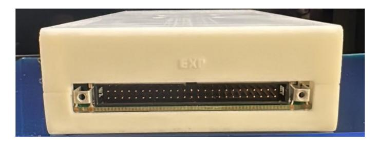
Expansion Connector – For adding expansion boards to the OSSC Pro. Expansion boards can add new functionality and input and output options.
