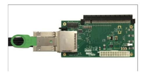
Connect the other end of the cable to the host adapter card.
