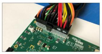
Connect power to the PSU and turn the switch to ON position. The "3AUX GOOD" LED comes ON.
