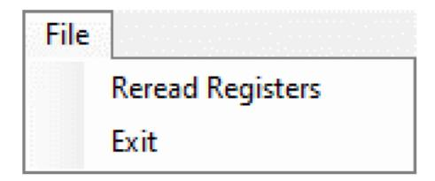
The Reread Registers function forces the program to re-read all of the control registers from the device and display them on the screen. This does not read the output data, because the program reads those registers continually while it is running. Click on the Exit command to close the main window and terminate the application. Any unsaved log data is cleared from memory. The application can also be closed by clicking the red "X" in the upper right hand corner.
