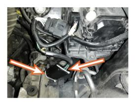
Mount the SMART CANBUS (load resistor) to the vehicle's body (metal). Please note: Pull the cable ties until they are taut. 6)
