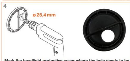
Mark the headlight protective cover where the hole needs to be drilled (13 mm from the center toward the right). Using a step drill, drill the hole needed for the cable to pass through. 3)
