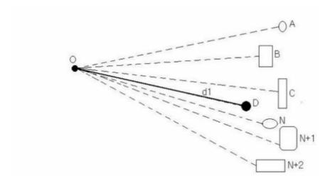
In the pinseeker mode, the point D may be isolated from a number of points in the background and keep only the distance d1 to the point. This is done to achieve automatic locking distance.
