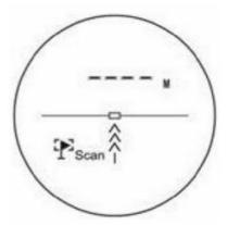
**Model P:** Press power button shortly, the distance value will display. Long press power button, it will start continiously measuring around flagpole until the value is stable. This value is the distance to flagpole.
