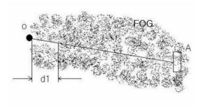
Fog can reflect the laser generating, so when it's fog, it's hart to measure distant targets. Filter out fog errors caused by distance (d1=30m), ensuring long-distance measurement volume.
