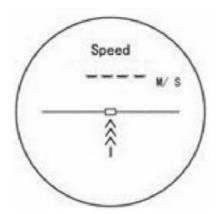
**Model P and H:** Target the moving object and press power button shortly, and keep on targeting the object until the speed value displays on the screen.
