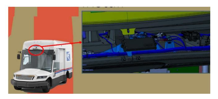
The antenna is mounted inside the center of the overhead console. **Cable length**: 159 inches (4033 mm) TCU to back of the Antenna.
