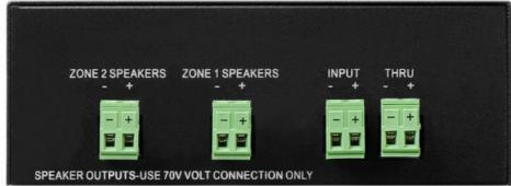
The SS2V70-200W is a unique 70V Speaker Selector featuring 2 independent Zones each controlled by a 200 Watt 70V Mono Volume Control featuring a Rotary Style Knob. Each zone has On/Off switch as well. The unit has a single 2 conductor input and direct pass through allowing to stack additional SS2V70 Speaker selectors only limited by your application. Standard 70V rules apply to the number of speakers used per zone, matching the available power from the 70V amplifier.
