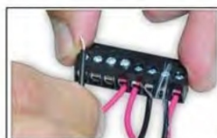
Loosen the set screws for each conductor
